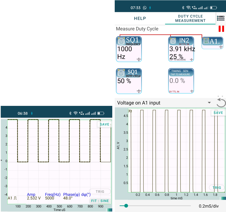
Figure 4.3: (a) Squarewave on TC0 (b) PWM waveform on TC0
