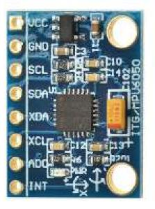
I2C module with Accelerometer, Gyroscope and Temperature sensor
