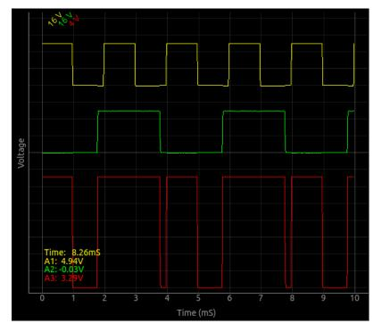
The results for the AND gate made using the IC 7408 is shown below.
