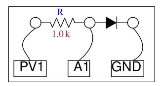
• Make the connections as shown in the figure. Use  $1000\Omega$  resistor
