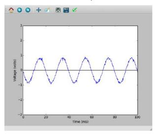
The amplitude of the pickup depends on the wattage of the electrical equipment operating nearby, distance to them and on the length of the wire used.
