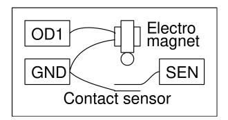
• Attach the iron ball on the electromagnet
