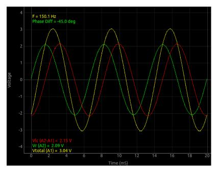
The next step is to study the RL circuit. Here you will observe the current waveform lagging behind the voltage across the inductor.
