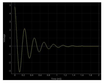
The values chosen are for an underdamped response. The coil has in inductance more than 100mH and a resistance of around  $500\Omega$ . To increase damping, you may add a series resistor, or use a larger value capacitor.
