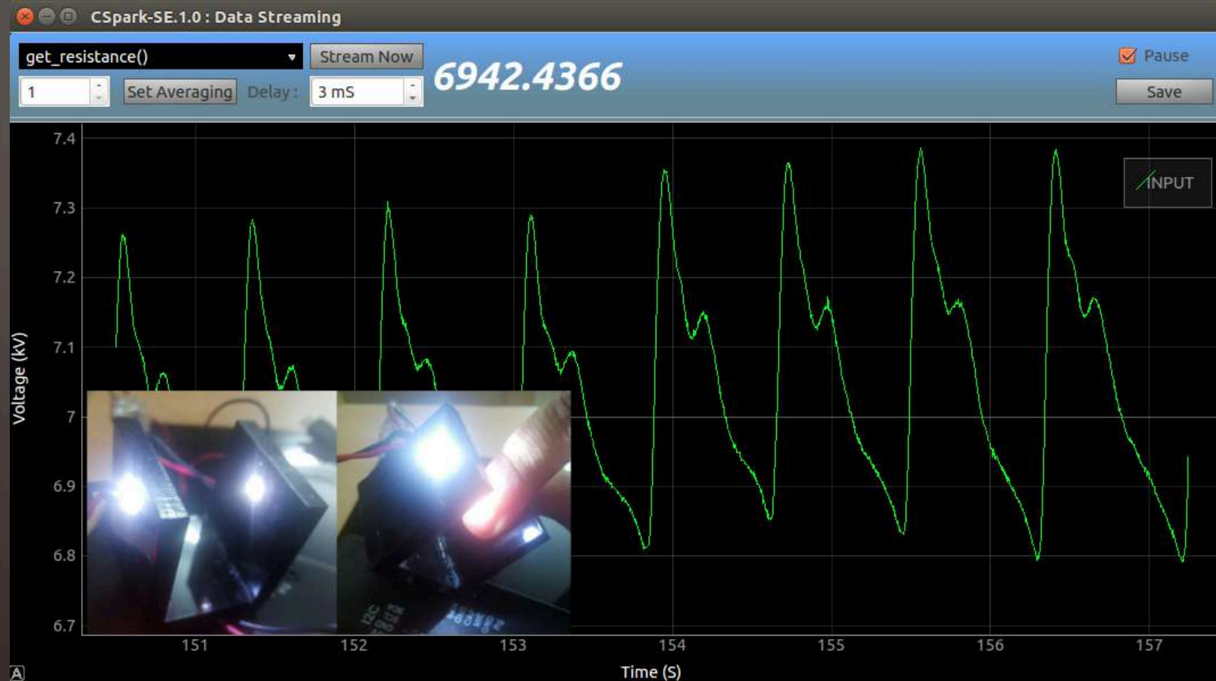
Heart rate detector with the Data logger, an LED, and a phototransistor
